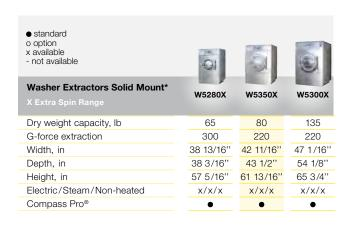
Soft Mount machines Direct installation on all types of floors Solid Mount machines Need to be bolted to concrete pad
